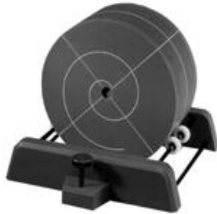
Figure 10: Solid water phantoms used in quality assurance tests, solid water slabs, and a cylindrical phantom
