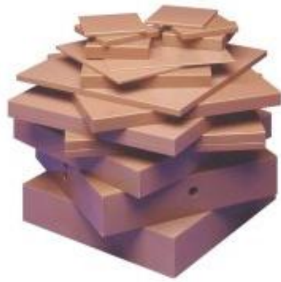
Figure 10: Solid water phantoms used in quality assurance tests, solid water slabs, and a cylindrical phantom
