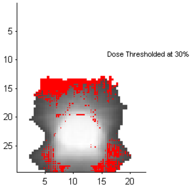
Figure 37: Gamma Pass/Fail diagram for Rando Prostate patient 6 using a 3mm DTA and 3% dose difference tolerance. The analysis region was defined as the area of film receiving over 30% of the prescribed dose.
