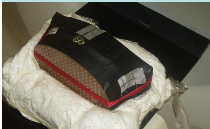
Figure 15: The Pelvic and Lung phantoms used in the RANDO phantom study. The pelvic section consisted of slices 26-35, and the lung section consisted of slices 14-19.
