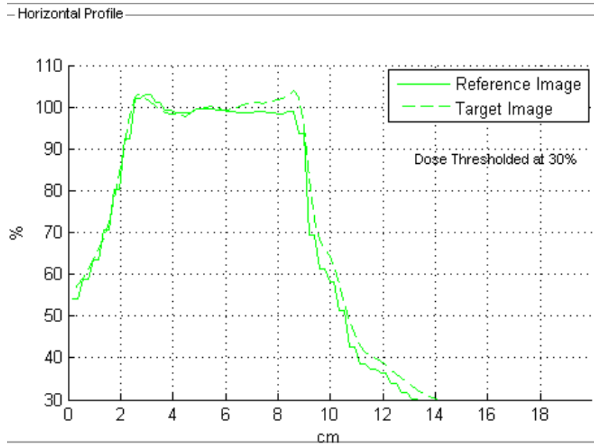
Figure 52: Horizontal and Vertical profiles for RANDO lung patient 9. Horizontal and vertical profiles spatially evaluate the dose distribution between the calculated and measured profiles.
