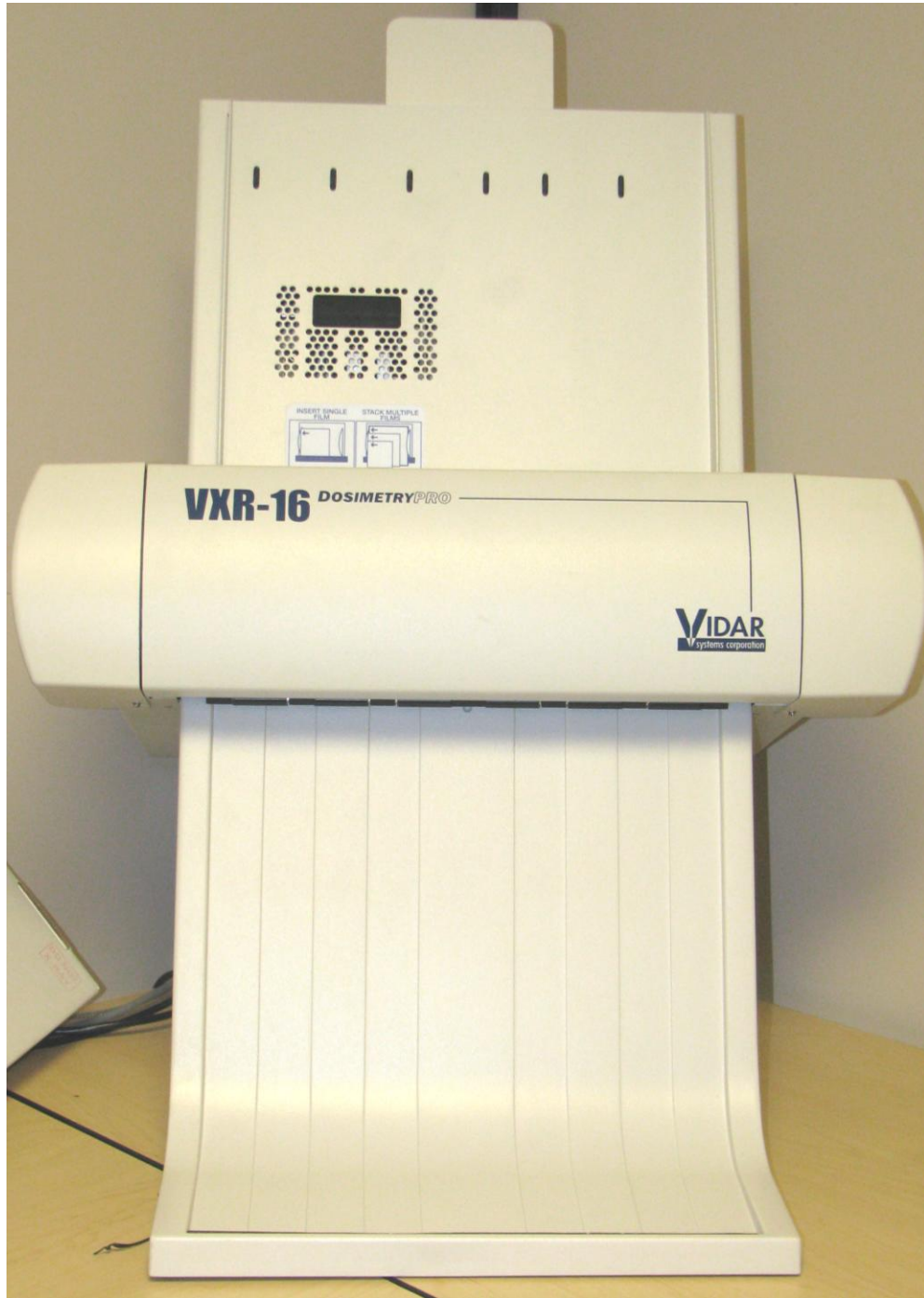
Figure 17: The Vidar 16 Dosimetry Pro at the Thompson Cancer Survival Center used to scan the processed films.
